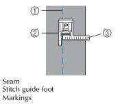
Aligning the fabric with a needle plate marking The markings on the needle plate show the distance from the needle position of a seam sewn with the straight stitch (left needle position). Sew while keeping the edge of the fabric aligned with a marking in the needle plate. The distance between the markings in the upper scale is 1/8 inch (3 mm) and the distance between the markings in the grid is 5 mm (3/16 inch).
